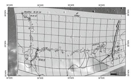
Fig. 9 Differences between Lunokhod-2 route, digitized in GIS (white), and the route from transformed historic topographic schema (black), produced as the result of analysis and mapping after Luna-21 mission (maximal discrepancy, marked with arrow, is about 80 m)
