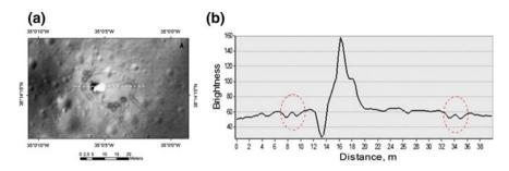
**Fig. 3** Analysis of brightness of Lunokhod-1 wheel tracks: (a) LROC NAC image M175502049 with resolution 0.3 m/pixel; (b) corresponding profile of brightness along transect line with white dashed color on the image. *Note:* W-shaped pattern on the plot representing tracks of left and right rover wheels
