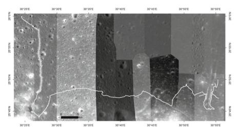
Fig. 4 Orthomosaic with high quality of visible track, produced to identify the route (equidistant cylindrical projection with center at study area—central meridian 30°40', standard parallel 25°50')
