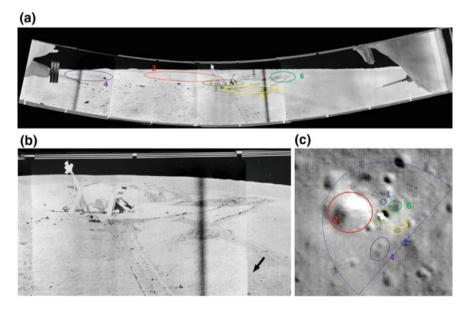
**Fig. 6** Implementation of Lunokhod panoramic images for identification of the wheel tracks: (a) Lunokhod-2 panorama #6-375 with marked prominent features that are also visible in LROC NAC orthoimage; (b) zoomed in fragment of the panorama—the ninth wheel track is marked by an arrow; (c) LROC NAC orthoimage of the landing site, observation point of the panorama is marked with a star
