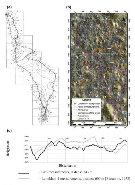
**Fig. 7** Topography for the southern part of the Lunokhod-1 traverse area: (a) topographic map from Leonovich et al. (1978); (b) contour map, derived from LROC NAC data; and (c) comparison of profiles for the part of traverse (blue line at the contour map)
