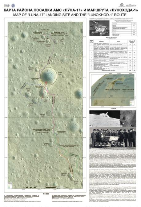
Fig. 10 Map of the Lunokhod-1 route (Karachevtseva et al. 2016). Original size of map sheet is  $594 \times 841$  mm. Colors of route parts show distance travelled through single lunar day
